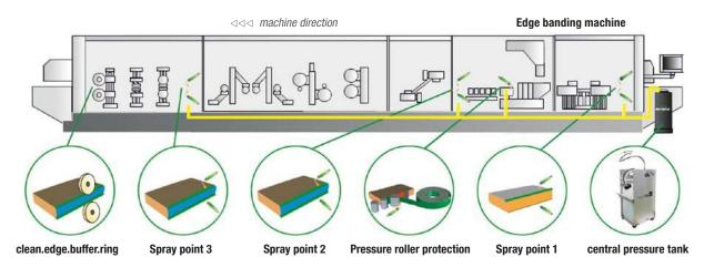
One Liquid for the entire working process. clean.edge.liquid HP acts as a separating agent, coolant and cleaner.
